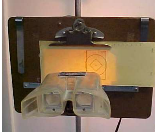
Figure 2.5. This stereoscope was originally purchased from Keystone Corporation and was modified by the author to allow the patient to stand while using it. It can be raised or lowered on the pipe in the back to adjust to children or adults. The Cheirosopic tracing test target is shown here with the printed picture centered in front of the left eye. The tracing would be done first with the right hand and the right eye viewing the pencil with the left eye viewing the picture.
