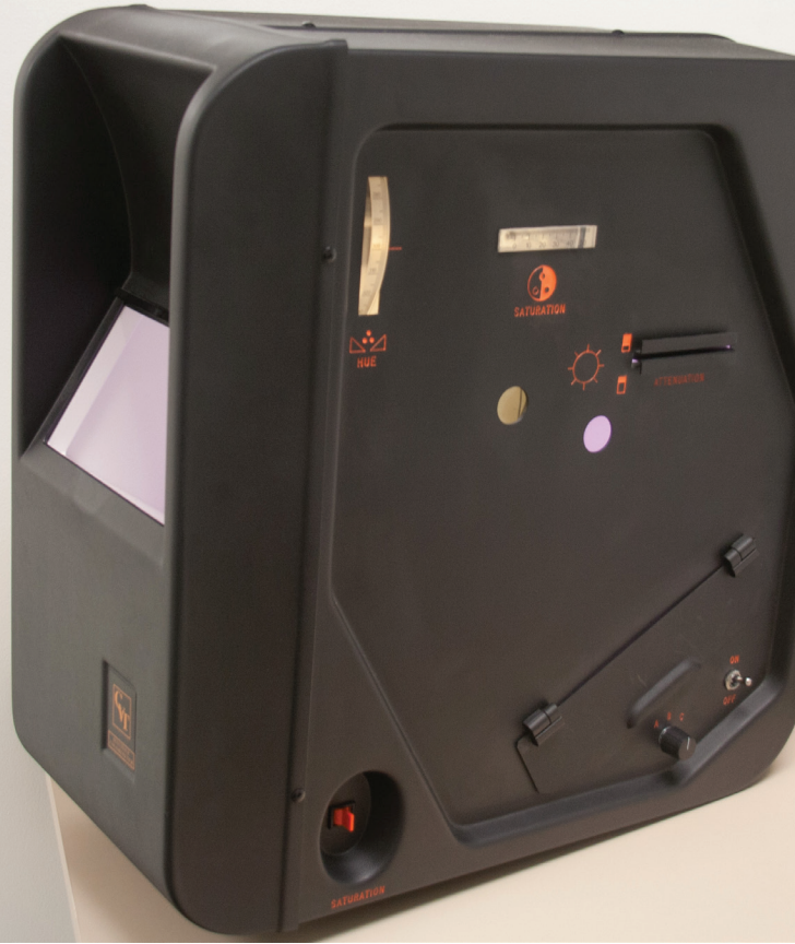
Figure 3 shows the saturation adjustment used. "0" represents white light and the light is the same at the "0" setting regardless of where the hue wheel is set. When the saturation is set at any other number some color is clearly seen. At the "50" setting the color is seen as saturated as the device is capable of showing.
